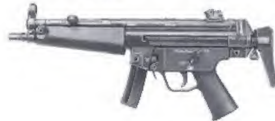
Fig. 2 MP5-N with butt stock retracted
